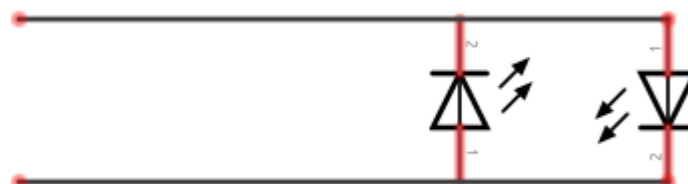
Figure 3 Connection diagram of indicator LEDs
